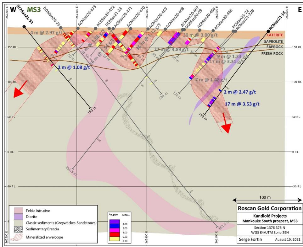
Figure 2: Cross Section Depicting East Extension at MS3 – RCMa21-55
